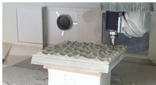
One panel being CNC milled (Image: Peuckert)
