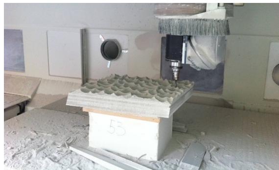
Each panel was manufactured on a milling-machine according to Benjamin Samuel Koren's input. © Peuckert
