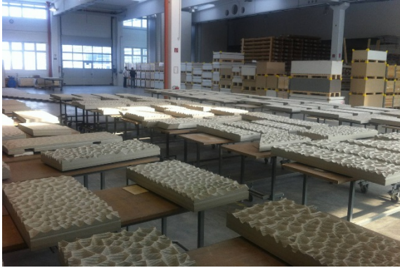
The Bavarian company Peuckert manufactured the panels according to the specifications coming from Frankfurt - 10,000 files for 10,000 panels. © Peuckert GmbH
